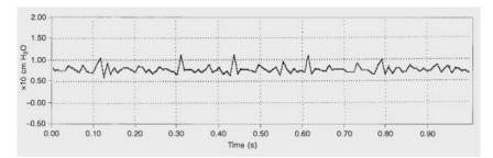
Waveform produced at airway with bubble CPAP. Flow set at 8 liters/min; amplitude of waveform 2–4 cm H2O; waveform frequency approximately 15–30 Hz
