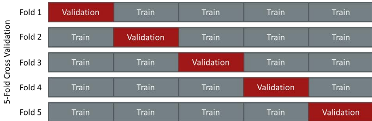
Figure 6. When large amounts of data is not available k-fold cross validation can be used. Five fold cross validation is shown here. In fold 1, the first sample is held for validation and the other four sets are used for training. In the other folds different samples are used for validation. The cumulative error for k-fold cross validation is the average error of all the folds.
