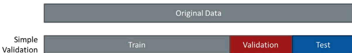
Figure 5. With a large amounts of data simple validation can be used to divide the data into three parts. The training data (50-60%) is used to develop the model. The validation data (20-25%) is used to determine performance and error during development. The test data (20-25%) is held until the end to assess generalizability of the model.
